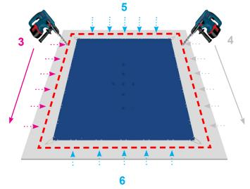
Drill then install by following the order shown on the diagrams.
