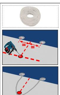
Drill then install by following the order shown on the diagrams.
