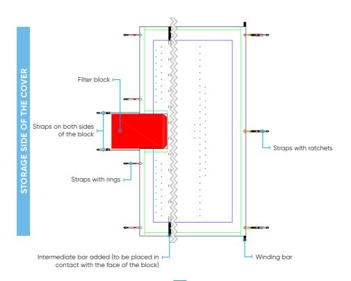
In the case of a block on the opposite side to the storage side (the side where the winding bar is located):
