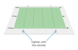
Tension the straps passing through each bar of the cover.
